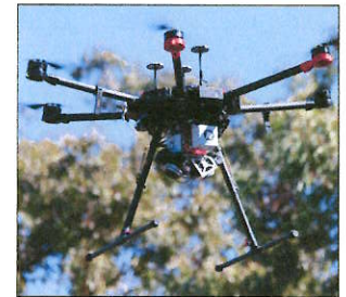
DJI Matrice M600 equipped with RIEGL miniVUX-SYS using RIEGL Integration Kit 600
