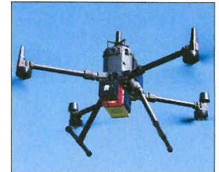
DJI Matrice M300 RTK equipped with RIEGL miniVUX-SYS using RIEGL Integration Kit 300
